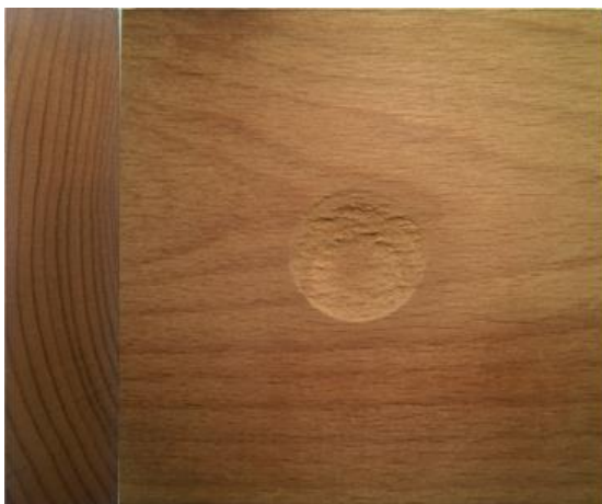
Figure 9: Heat treated beech sample after sandblasting
