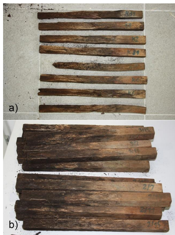
Figure 23: Unimpregnated (a) and impregnated (b) beech samples after 18 months of soil contact
