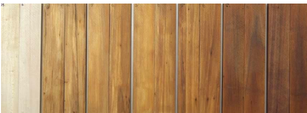
Figure 13: Colour change of poplar wood due to different heat treatment schedules in linseed oil
