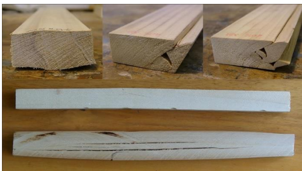
Figure 19: Typical failures of poplar wood as a result of THM treatment
