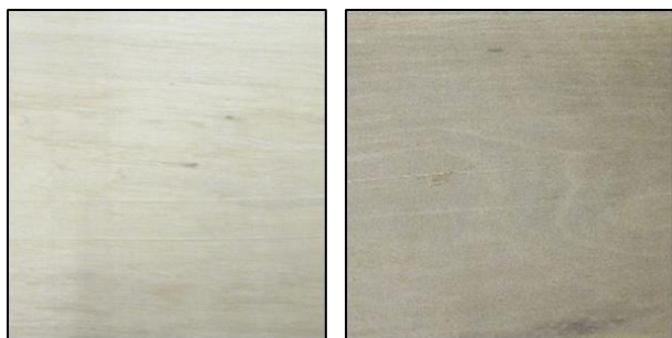
Figure 22: Colour change as a result of acetylation on hornbeam wood (left: untreated; right: acetylated)
