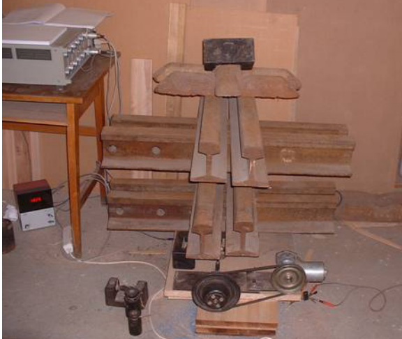
Figure 3 – Shifting a weighed-down workpiece on the raster table
